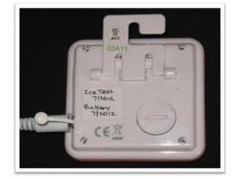
Record the date of when Battery <u>changed</u> and ice slurry preformed on the Min/Max thermometer.
